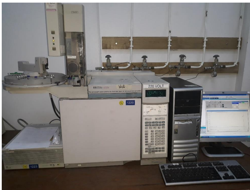
Figure 24. Hewlett Packard HP 6890Series Gas Chromatography instrument, with a Flame Ionization Detector, at the Polytechnic College (PTC).
